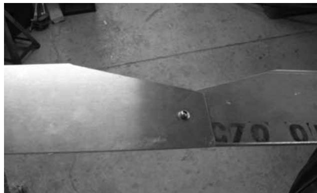
rivets in this area. Simple logic would say this plate could take at least a 4800lbs of shear load from the main spar bolt, though this would not be the case as loads would be supported by other components. The area of each gusset would actually see about  $\frac{1}{4}$
