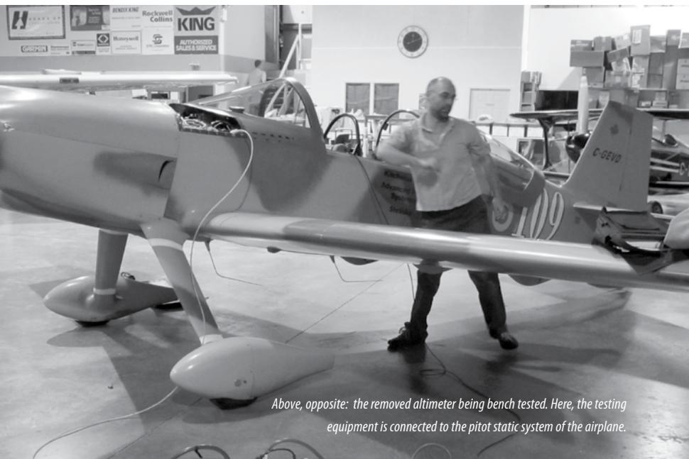
*Above, opposite: the removed altimeter being bench tested. Here, the testing equipment is connected to the pitot static system of the airplane.*
