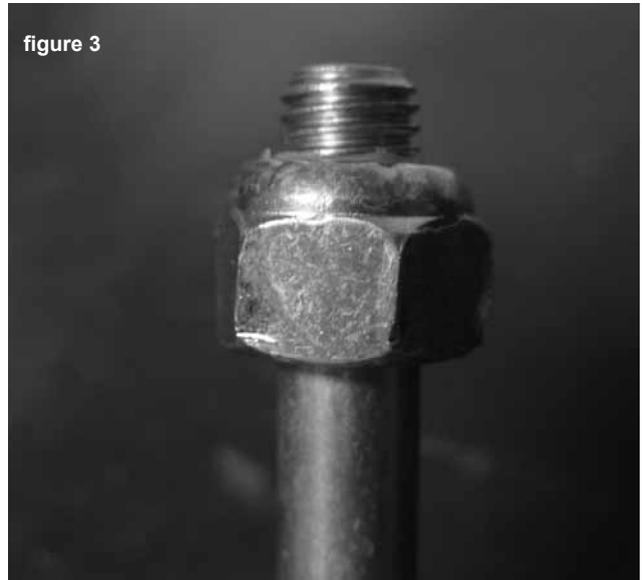
threads will grip the bolt. Others have the end of the nut squeezed into a slightly oval shape, and as the bolt screws up through the threads it must make the hole round. This provides gripping action.
