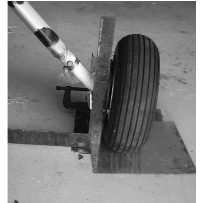
Above left: My Rocket has a tapered aluminum spacer between the gearleg and the bolt on axle. I was lucky that by rotating I could use the same spacer. Otherwise I would have been off to Spruce or to a friend's machine shop for a custom part. Right: Camber can be checked with a framing square. The grease plates have moved quite a lot during the iterations of the test. If they pick up grit they will stop sliding, so keep the floor clean
