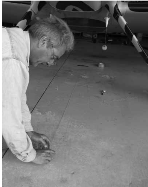
Left: Tape the string to the rearmost point and extend it forward, crossing the forward point. Below, left, sight down the rim or disc and set the straightedge on the floor. Below, measure the distance to the centerline at both ends of the straightedge. One inch difference over 5 ft is 1 degree.
