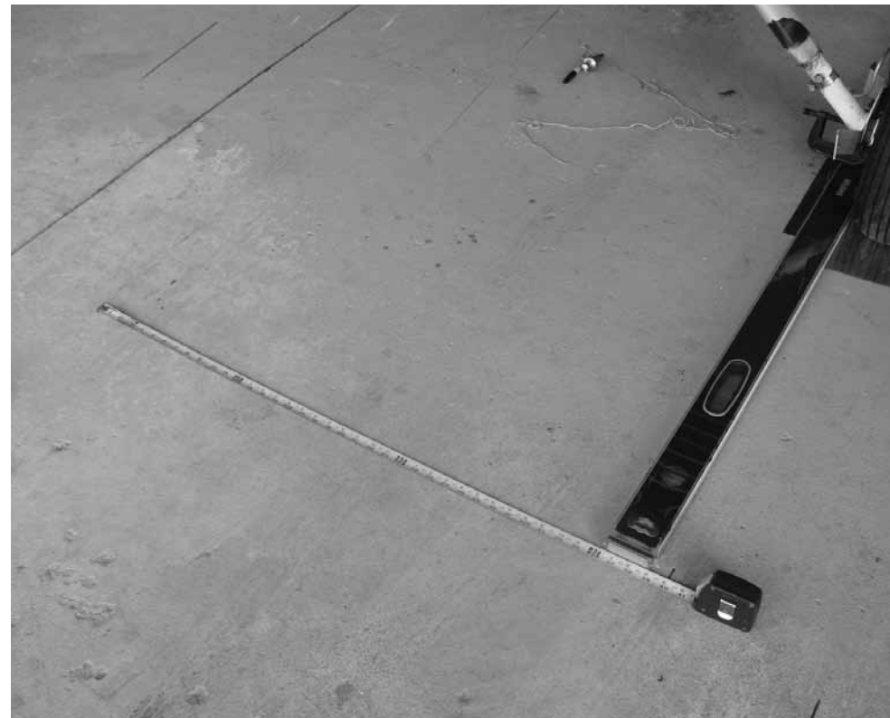
Left: Tape the string to the rearmost point and extend it forward, crossing the forward point. Below, left, sight down the rim or disc and set the straightedge on the floor. Below, measure the distance to the centerline at both ends of the straightedge. One inch difference over 5 ft is 1 degree.
