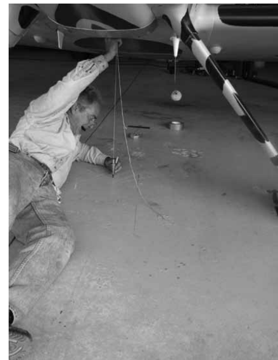
Top: Jack the gearleg up and spin the wheel to check trueness. If the bearings are loose, snug them up for the measuring. Left, Using a plumb bob mark centerline points on the floor. Note the tennis ball on the tip of the antenna.
