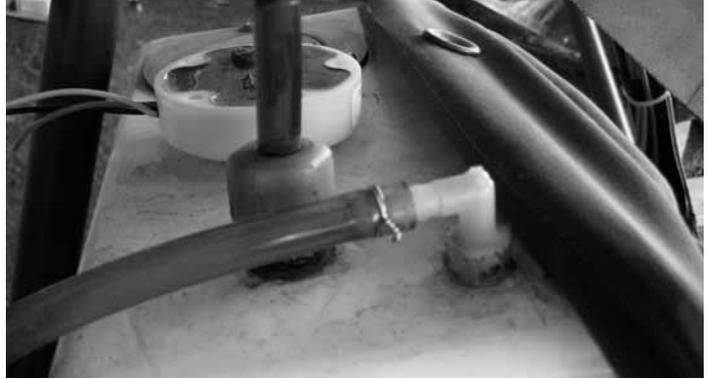
Have you ever needed another hole in your gas tank for a supply line or vent line?? Here is a simple way to achieve that goal. I am installing this so my suction line for my primer is not teed into my main fuel line. The following picture is of the original vent elbow (Right, top).
