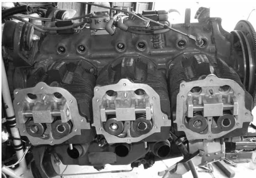
From the top down: Installing cylinder and piston on the connection rod; Removing the piston pin; The cylinders in place
