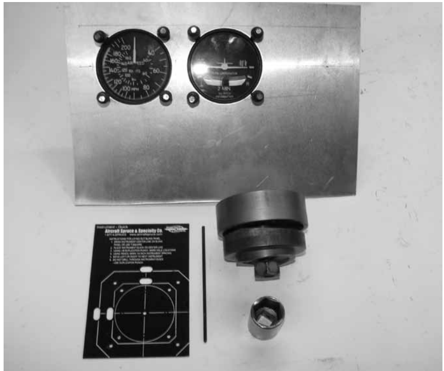
Above, The Spruce gauge template and the ATS panel punch
