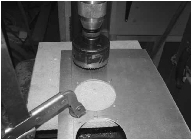
Left, A good holesaw does an effective job if the panel is backed up and clamped Right, a shop made template will aid in laying out the Kollsman adjuster hole
