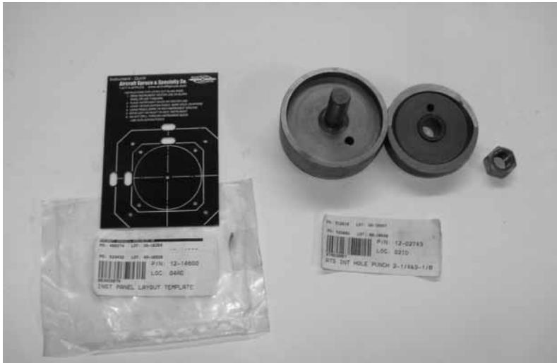
Top: The Spruce gauge template and the ATS panel punch. Left, the transfer punch is used to lay out the hole centres. Right, do not drill through the template or you will lose its accuracy. Left, test panel with template and tools.
