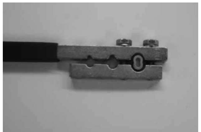
Top left: First test swage is the centre one...and results in a little bow tie (above). Top right: Check the swage with the go-no go gauge. Lower right: Forming a thimble eye begins with centering the Nico and squeezing just enough to trap it in the jaws.
