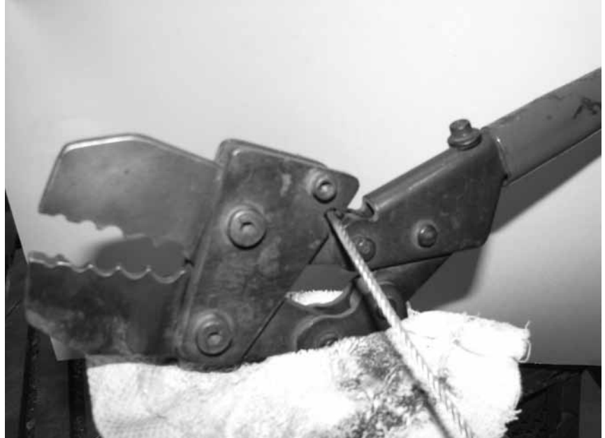
Top left: A thimble eye loop in 1/8" cable, formed with the Swage-It AC 43-13 requires three squeezes with ridges between each, with a little ridge each side. Lower left: Prepare the thimble by spreading the tips to ~.100° separation. Above, begin by cutting some test pieces. The $350 swagers include a cable cutter.
