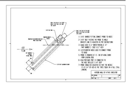
THE "LIFT RESERVE INDICATOR" has been referred to as an angle of attack meter, a lift management system and an air speed system. It is probably all of the above.
