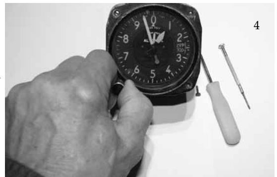
Fig 2: insert a paperclip or a small screwdriver into the threaded hole and slide the pin outwards. It will probably be stiff, but it will click and move 1/16". This frees the adjusting knob.
