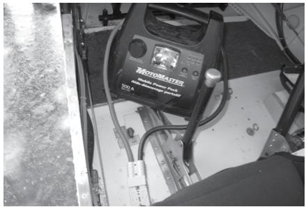
One man boosting: when you don't have someone handy to hold heavy wires run from the battery to a welding cable connector under the pilot's seat. The matching connector is attached to the booster pack. When you are ready to boost your battery simply retrieve your booster pack from your gear, start your engine and let it warm up while you re-store your booster.
