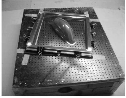
Top: the perfect shape for the lense. Centre, left, the mold taken off the bottle, and right, the plug made off of it. Note the pegs that position it on the pegboard. Meticulous finishing is necessary - the smallest flaw will be visible on the finished lense. Above: the vacuum frame which was connected to a shop-vac. All the holes outside of the frame area were sealed with clear packing tape.
