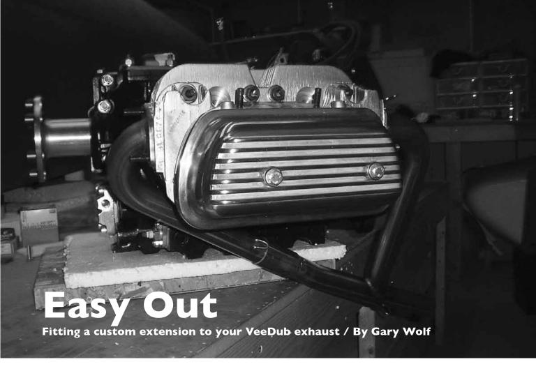
AEROCONVERSIONS SELLS a welded stainless exhaust system for VW engines and it is nicely made but requires that the exhaust studs be removed to install the system. A member brought in his brand new Aeroconversions exhaust system for some advice on how to mount it on his Sonex.
