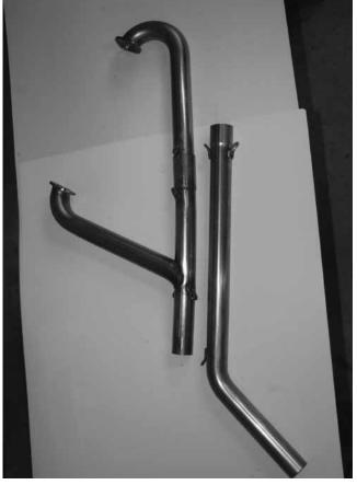
Top left, the exhaust **must** be bolted to a head while being welded.
